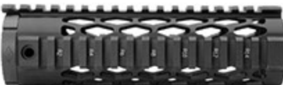
HG1094 YHM Diamond EXT Features diamond shaped heat vents, an extended top rail for gap-free installation, "T" marked rails, and anti-rotation screws. Hard cast aluminum and hard coat anodized. Price: $122.70
