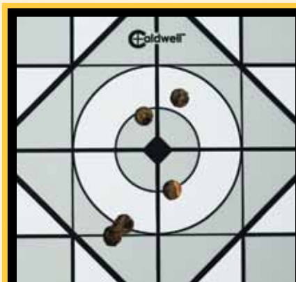
This rifle had zero malfunctions and proved accurate with all types of ammo, producing 2-MOA or better groups.
